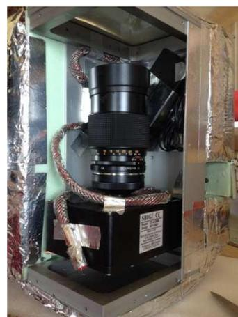
Left: tests on the pointing system observing SuperDARN container (upper-right image on the screen) – Right: CCD camera with heating cables and foam insulation.
