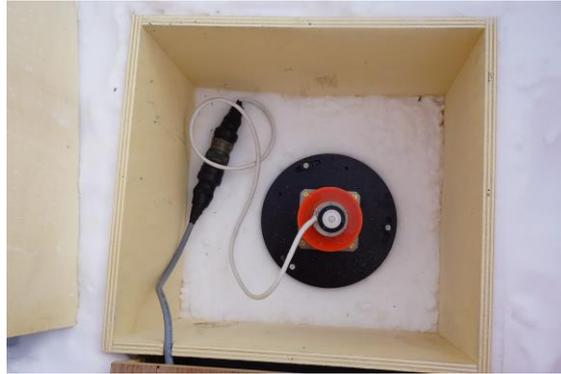
Figure 3. Flux-gate magnetometer sensor installation
