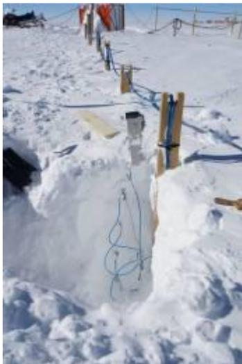
Fig. 1 – The snow temperature probes realigned to their nominal depths
