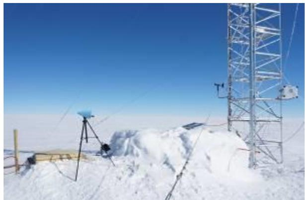
Fig. 3 – The spectrum analyzer antenna mounted on a tripod measuring RFI from the American tower (on the right) towards the Station.
