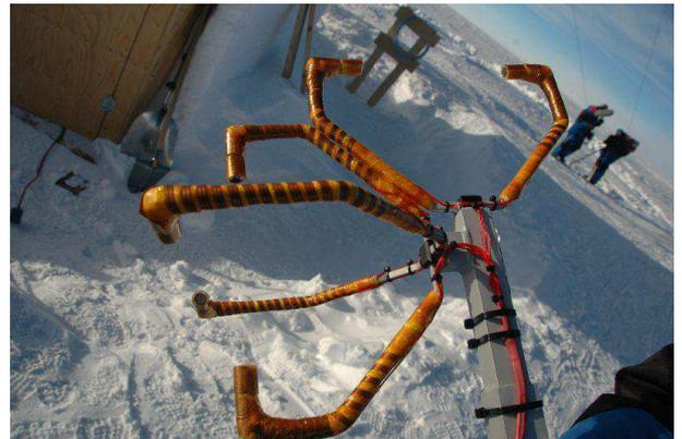
Fig. 5. A sonic anemometer (Photo E. Aristidi)
