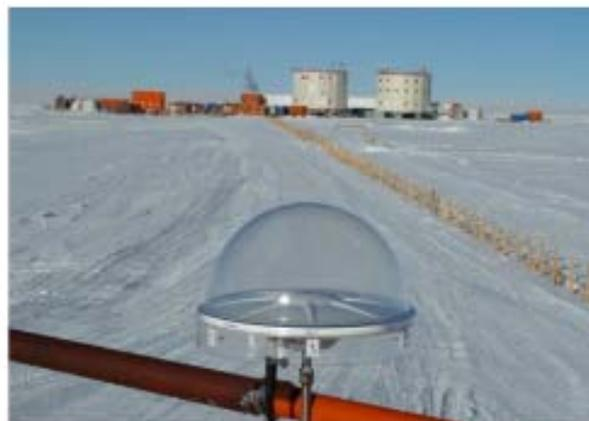
Installation of a GPS on the roof of the HAMSTRAD shelter in order to get IWV on a quasi real-time scale, hopefully next year
