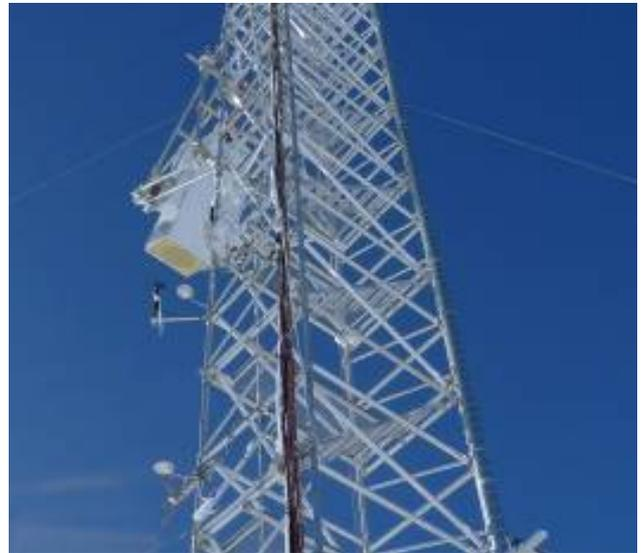
Fig. 2.6 - The L-band radiometer placed on the American tower
