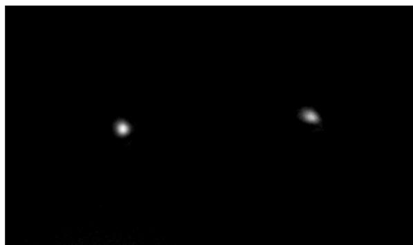
Fig. DC.4 - Left, the DIMM system. Note the 2 hole mask at the telescope top. The box at telescope back contains the camera. Right: typical short-exposure frame of the star Canopus at the focus. The two images move with turbulence, analysis of their differential motion provides the seeing.
