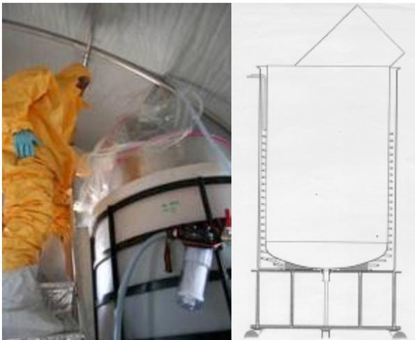
Fig. DC.2 - The new experimental device used during the 2005-2006 field expedition: a stainless steel double tank clean snow smelter working together with a 35kW propane boiler. The melted snow is sieved through a 30µm mesh at the bottom of the smelter.
