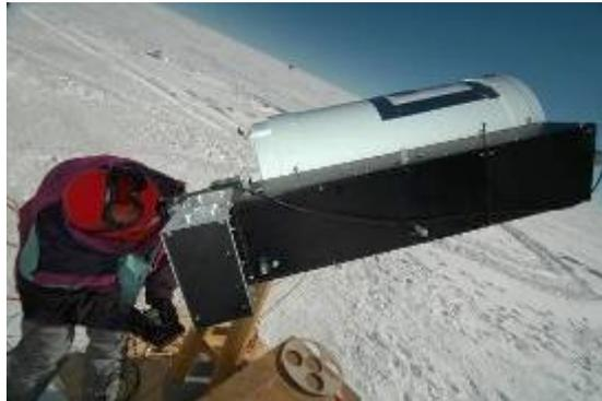
Fig. DC.10 - The Corona optical bench (the black box) fixed on a Celestron 14 telescope.
