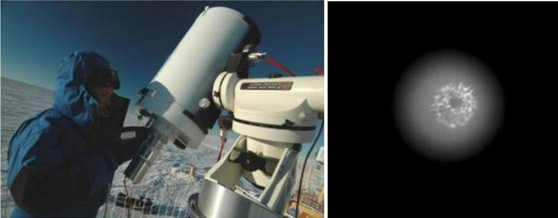
Fig. DC.9 - Left: The SSS at the focus of the Meade 16 telescope. Right: First image of a defocused star through the SSS obtained on January, 15<sup>th</sup>.
