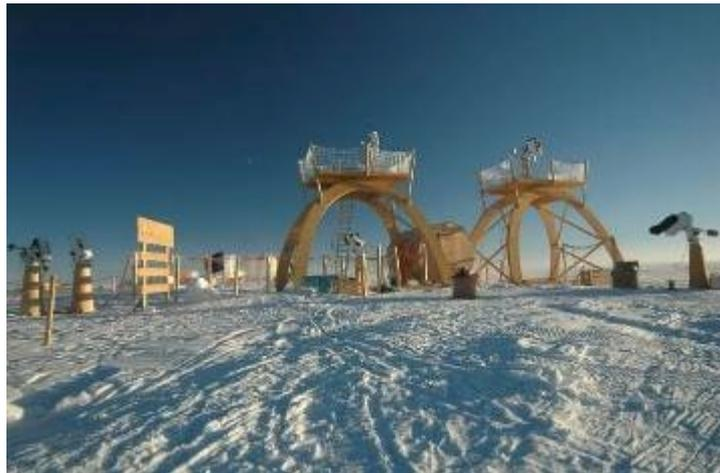
Fig. DC.3 - General view of the ConcordiaAstro observatory in January. Twin telescopes on the left are the GSM experiment. The DIMM is on the left platform, the SSS is on the right one. Corona is the telescope on the ground on the right. Notice the wind screen in front of GSM.
