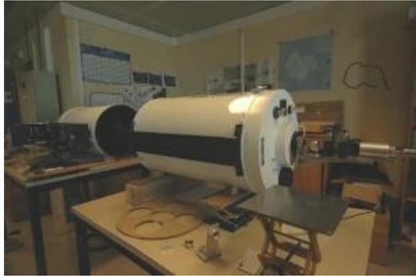
Fig. DC.11 - Left: The optical bench made of two telescopes facing each other.
