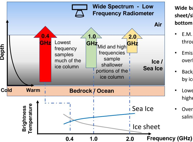
Wide band radiometer 2 Possibility to observe ice sheet/shelves/glaciers/sea ice from surface to the bottom
